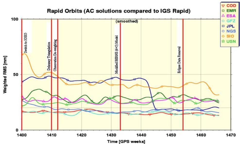
**Fig. 4** Time series of Weighted RMS taken from the IGS Final orbit combination for each contributing IGS Analysis Center. A red, vertical line marks the epoch at which a change in processing strategy was applied. NGS is shown with a medium blue line and medium blue circles. Plot adapted from <http://www.gfz-potsdam.de>
