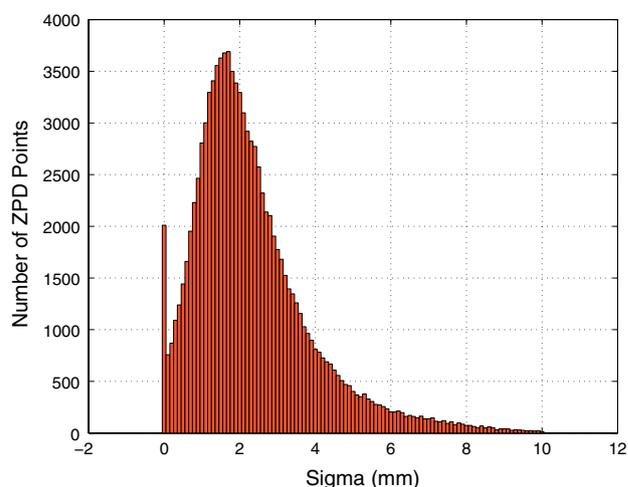
**Fig. 2** Histogram of the formal errors reported for the legacy combined final troposphere solutions. The histogram was generated using 30 site solutions for year 2003. Zero sigma is reported when only one AC contributed a solution for a given site
