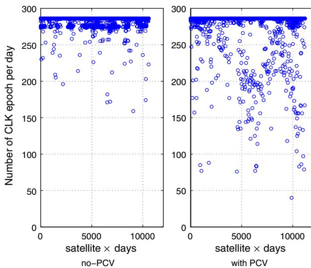
**Fig. 9** The number of clock epochs in the IGS clock files for each satellite, during 1 year before November 2006 (no-PCV) and 1 year after November 2006 (with PCV). The *x*-axis denotes the satellite  $\times$  day ordinal number during the 1 year time span ( $365 \times 30 \approx 11000$ ); Note the significantly increase in number of missing epochs after the transition to PCV modeling
