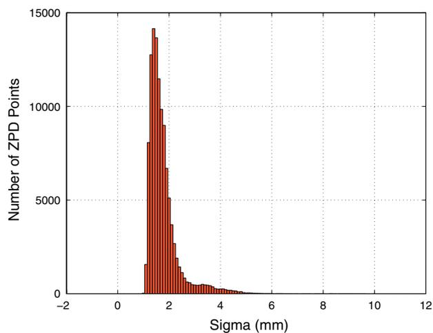
**Fig. 3** Histogram of the formal errors reported for the new Final troposphere product. The histogram was generated from daily precise point positioning for a set of 30 globally distributed sites for year 2003
