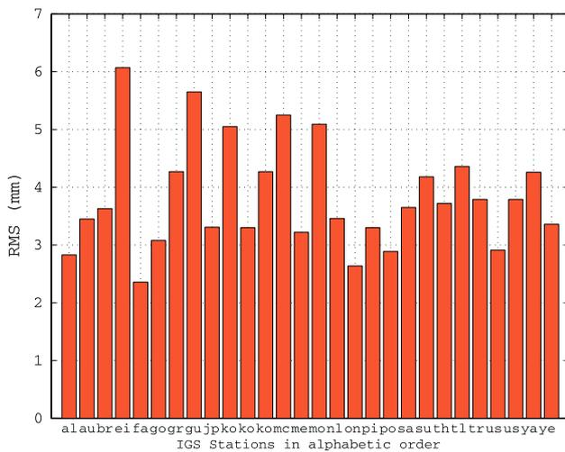
**Fig. 4** The RMS of ZPD differences between the new and legacy strategies for each site selected for the comparison. *x*-axis denotes the station list in alphabetic order; *y*-axis denotes the RMS of the ZPD differences in mm
