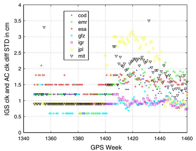
**Fig. 10** The standard deviation value of difference between IGS combined clock solution and each AC's clock solution are extracted from IGS summary files from GPS week 1348 to 1460. This period spans 2 years with GPS week 1400 at the center. The *x*-axis denote the time in GPS week and the *y*-axis denote the standard deviation of clock difference in cm
